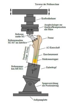
Figure 2: Fatigue tests of hip endoprostheses
