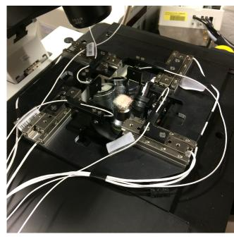
Device for biaxial extension tests (Pukaluk et al., 2022)
